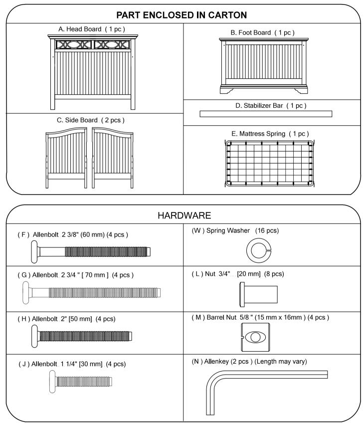
Make sure the bolts are tightly locked against the washers during assembly. (Please add an extra ½ revolution to all the bolts when using spring washer after tightening)
