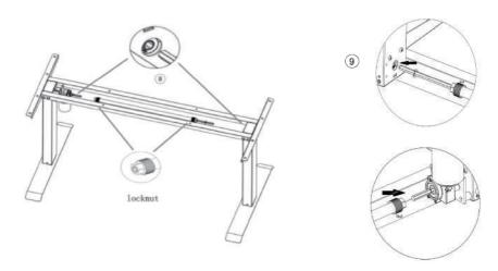
Install the frame on the desktop. Then install the K -AC Adapter.
