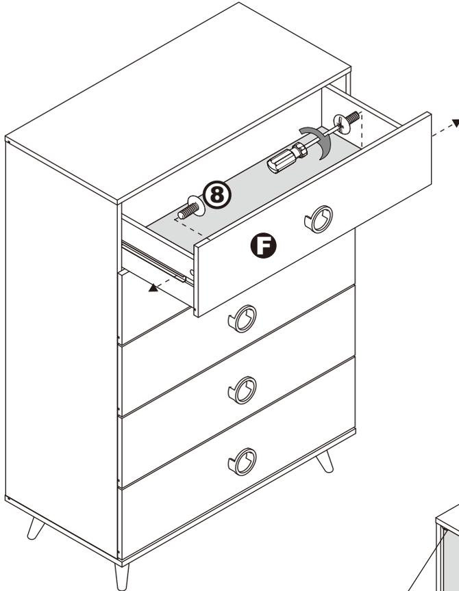
Extend the two outer slides of the runners so that they could align with the sides of the drawer. Make sure the pre-drilled holes from the drawer align with the screw holes of the outer slides.
